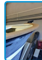
PVC 2441T Top side gunnel profile 120mm wide Minimum order quantity
